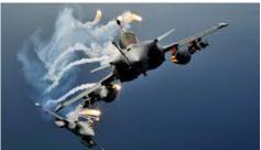
SPECTRA comprises Infrared (IR) Missile Warning System, a dedicated management unit for threat level assessment and multi-threat decoy dispensers with a smart dispensing facility. System facilitates Rafale a high survivability against a range of airborne and ground-based threats.
