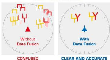
Implementation of the "multi-sensor data fusion" in Rafale facilitates accurate, reliable tracks, uncluttered displays, reduced pilot workload, quicker pilot response and a clear situational awareness. The automated process is carried out in three steps with advanced signal processing coupled with in-built library.
