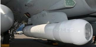
TALIOS has high-resolution sensors and high-precision line-of-sight stabilisation with wide-angle vision providing critical contextual information and making the pod a key component of the pilot's visual environment throughout the mission. It was developed in an open architecture conceived as a 'plug & fight' system with a high level of functional integration.
