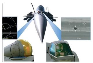
The FSO is developed by M/s Thales. The system operates in the optronic wavelengths and hence immune to radar jamming/ECM. It also provides covert long-range detection and identification, high resolution multi-target angular tracking and laser range-finding for air, sea and ground targets.
